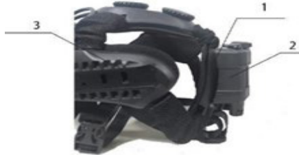
FIGURE 2.16 CONNECTING THE EXTERNAL BATTERY BOX TO THE HELMET
