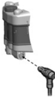
FIGURE 2.14. CONNECTING THE CABLE TO THE EXTERNAL BATTERY BOX
