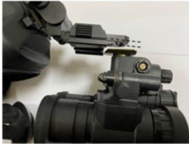
FIGURE 2.13. INSTALLATION OF HELMET MOUNT TO GOGGLES
