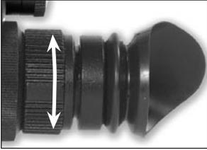
To focus the Patriot first you will need to adjust the diopter. Simply turn the diopter clockwise until it stops. Then, while looking through the diopter at a subject, slowly turn the diopter back counter clockwise until the grain in the image is sharp.
