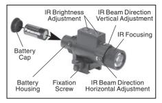
You can also change the position of the IR control panel fitting your needs. Undoing the small set screw on back of IR. Then use the included wrench to loosen back ring, Move the IR to its desired position/angle, retighten ring with wrench then retighten set screw.
