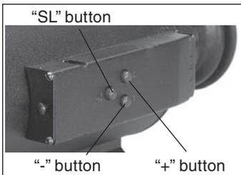
The scope will automatically shut down if it does not sense any activity for 20 minutes. Activity includes pressing any of the buttons or simply moving it back and forth away from your face. When activating the sleep mode the scope will first warn you by turning off the reticle for 10 seconds. If your intention is to keep using the scope, simply touch any key and the scope will reactivate.
