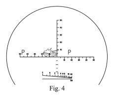
**4.2.2.B** When the azimuth of two targets is bigger than azimuth measuring range  $(-50 \sim +50 \text{ mils})$  inside the binoculars, on the target can be selected to make the necessary measurements in a step by step fashion. The sum of the
