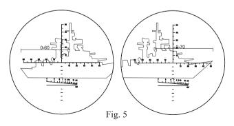
image where point B ended after the first reading. After calculating the mils for each image, You then can add them together to get the total azimuth read-ing. In the (Fig. 5) image below the ship is longer than the total 100 mils available on the reticle. However, by doing the foregoing mil calculations, you can now obtain the ship's total mil azimuth of 130 mils (60 + 70).
