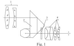
Basic binocular optical construction, as shown in Figure 1, consist of (1)the objective lens, (2) the erecting prisms, (3) the reticle and (4) the eyepiece. The reticle (3) is build in the right system.
