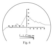
The value is the measured mils of angle included between the upper and lower parts. As shown in fig. 6, the value of the lower part is 40, the angle included between the upper and lower parts of the target is 0-75 (75mils).
