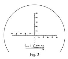
A mil's reticule can measure the azimuth angle, upper and lower angle, distance and size of an object or target. The visual distance reticule lines can measure the distance of normal object easily on the basis that the object to be measured is at least 2 meters (6 feet) in height.
