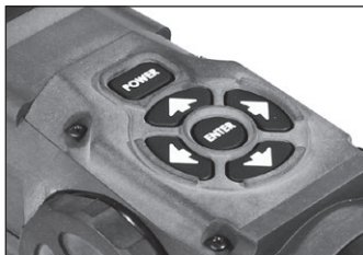
FIGURE 3.2. SWITCHBOARD OF THOR
