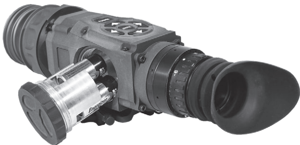
FIGURE 2.2. INSTALL BATTERY MODULE
